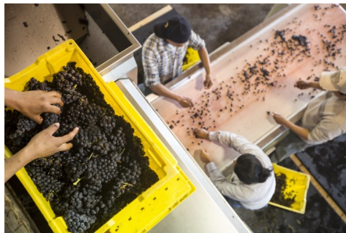
A worker loads grapes into mechanical sorting equipment at Delaplane Cellars; smaller stems and greenery are sorted by hand on a platform below. Logan Mock-Bunting /For The Washington Post
